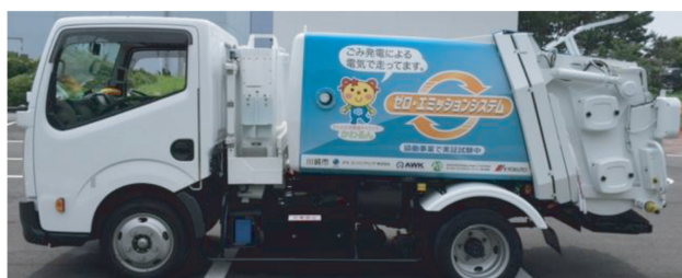
写真2 EVごみ収集車 Photo 2 ZeroE waste collecting vehicle with battery cartridge
